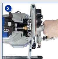
Remove pump section
