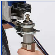
Open door and remove pump
