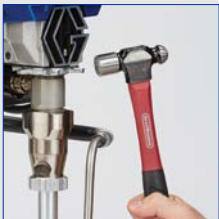
Loosen the clamping nut
