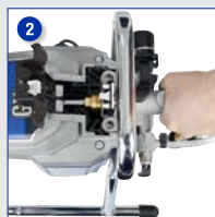
Remove pump section
